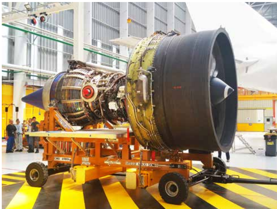
Special engine stand for engine test-cell use
